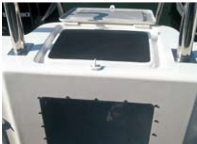
There is a fish hatch upfront on the deck with space for fuel cans on either side while there's also a cooler box hatch for the thirsty.
