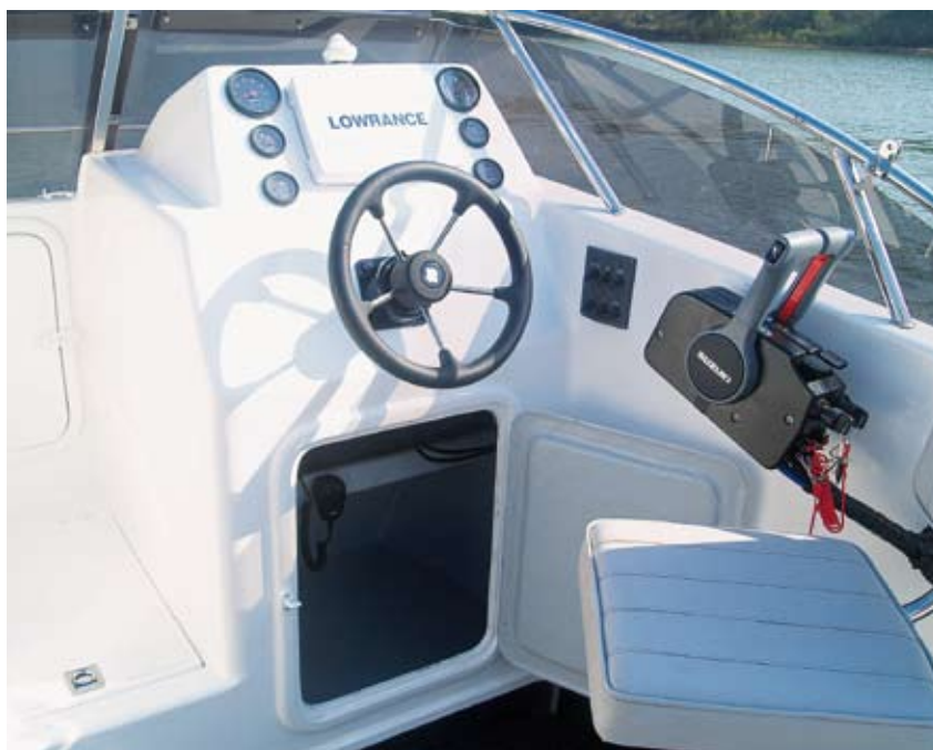
The Ocean Cat's impressive dash line-up includes two rev counters, trim/tilt gauges, compass, switch panel and Lowrance fish finder.
